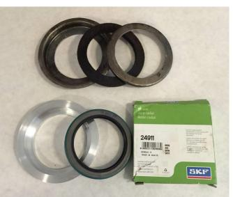
I'm not going to find a felt seal so option two how about a modern day neoprene seal. Down to Bearing Engineering with the old seal in hand and knowing I'll have to come up with some sort of adaptor. This seal SKF 24911 is my choice. With new seal in hand I call another friend and machinist Irwin Abrams to see what we can do to mount this seal into my wheels.
