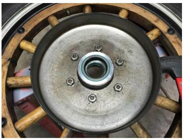
So step one repack the bearings with Marine grease while the adaptor gets cold. I'm not going to be able to pack them later. With the wheel on saw horses I tapped the adaptors into place and then the seals. I hope this is a permanent fix at least for my life time.
