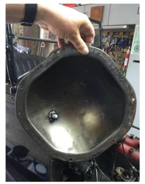
the rear end housi ng cover and found it clean no sludge but with a drain plug on the botto
